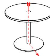
Wire management model has 4" dia. column and a step-up place beneath the work surface. Cable exits beneath the disc base.
