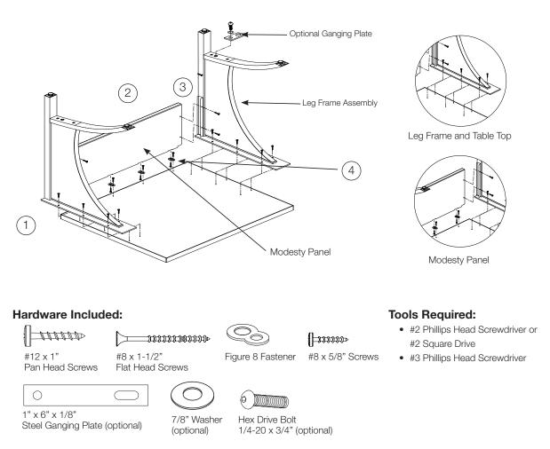
**Step 1**: To attach the leg frame assemblies to the table top, place the top upside down on a clean padded surface. Place the steel leg frame assemblies on to the table top above the machined locations. The U-channel that is fixed to the front post of each leg faces to the inside (one is right-facing and one is left-facing). Attach legs to the top using (6) #12 x 1" PH screws per leg. Leave the leg loose. DO NOT TIGHTEN.
