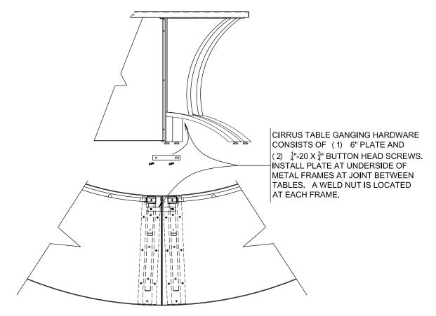
6" MENDING PLATE 400-066719-000 <sup>1</sup>/<sub>4</sub>"-20 X <sup>3</sup>/<sub>4</sub>" SCREW 800-000125-000
