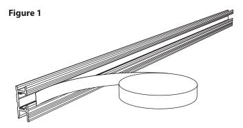
Slide the bottom edge of the fastener concealment vinyl into the screw channel located in the bottom of the center of the horizontal mounting track along the entire length of the horizontal mounting track. See Figure 2.
