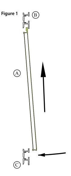
With upper and lower horizontal mounting tracks in place and properly installed, you are ready to "mount" elements Tiles.
