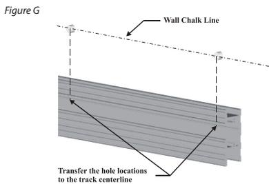
**Tracks must be straight, level and parallel.** Insure tracks do not "bow". Check for any gaps between the wall and the track and use spacers when necessary to shim between the wall and the track at attachment point(s) (Figure H). It is the responsibility of the installer and/or the contractor to select and install the proper fasteners in the structural wall. mediatechnologies® does
