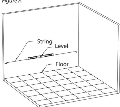
It is important that the string is tight and level for proper clearance of other components. Mark the location of string at each end. Snap chalk line using the two points defined above.
