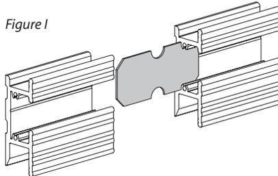
intersection, bend the Splice Plate to the required angle at the notch provided (Figure J).
