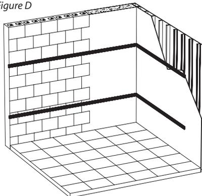
For proper attachment of track to the wall, fasteners must tie directly into the substructure of the wall (studs, blocks, solid masonry) (Figure D). Select the appropriate
