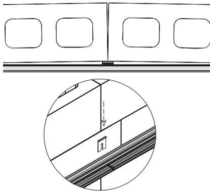
To align two adjacent pieces of track, slide a Splice Plate into the channel at the back of the track. Offset the "U" in the splice plate with the seam between the tracks (Figure I).
