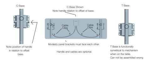
Flip application on welded or pre-assembled bases (handle release option shown).
