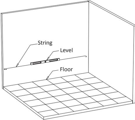
Several products are designed for the lower track. These products are mounted at 29" off of the floor.
