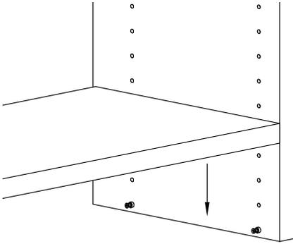
SLIDE SHELF ONTO THE CAM STUDS
